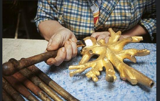
The finishing or «gilding» phase is performed by highly qualified specialists. We put extreme care into our finishing process and the final result is one of the most remarkable qualities of our products. Pieces are first "white pickled" in acid, then polished, de-greased, matted, treated with acid and sometimes varnished to better protect them against the ravages of time.
